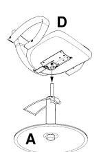
1) Locate the base with attached hydraulic foot
